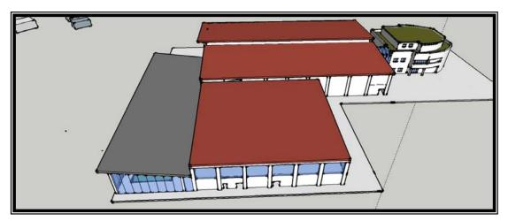
As can be seen below this development is focussed on maximising the use of the existing floor plan of the Arena with extensions being required to the south to accommodate the new swimming pool area and the north for the civic entrance
